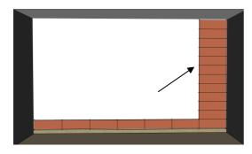
Continue to add pieces along your vertical reference line until finishing your vertical reference row. Keep the pieces edges straight and true to the reference line. When applying the last piece, keep the dilatation gap to the ceiling.
