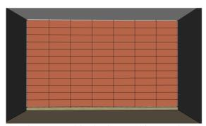
Continue to add planks working end to end keeping the joints staggered until the wall is complete.
