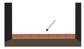
Continue to add pieces along your horizontal reference line until finishing your horizontal reference row. Keep the pieces edges straight and true to the reference line. When applying the last piece, keep the dilatation gap to the opposite wall.
