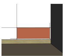
Install the first piece aligned to the horizontal and vertical reference line, in order to keep the necessary dilatation gaps.
