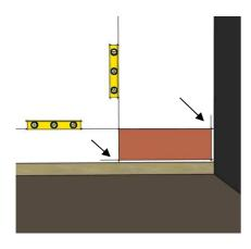
Draw a straight horizontal line and a straight vertical line on your wall to reference the first horizontal and vertical rows of pieces, always keeping a minimum distance of 1/4" for the wall and floor.
